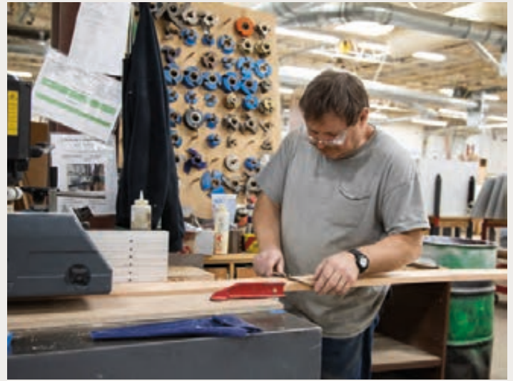
Mill Cabinet Local 51 member Dan Kubasek uses a shaper to form a bullnose decorative element.
